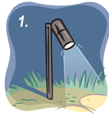
1. Barrel style directs narrow beam downward. 2. Mushroom head is effective on a flat elevation, not higher approaches.
