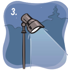
3. Low-watt flood is acceptable if pointed down, but scalloped-shroud design reveals lamp. 4. Pinholed mushroom head leaks a little upward decorative light.
