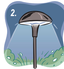
1. Barrel style directs narrow beam downward. 2. Mushroom head is effective on a flat elevation, not higher approaches.
